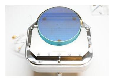
Image captions: A: Dielectrically coated 100mm diameter field selection mirror (courtesy: TNO).
